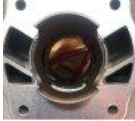
**136.8** check piston pin -- 0.420" maximum inside diameter
