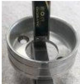
**136.4** remove head -- install dial indicator and using the LAD inspection tool -- check exhaust height (1.055") and inlet height (0.775")
