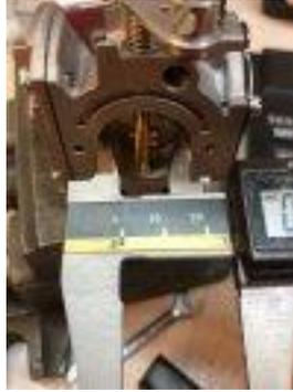
**136.2.2** remove carb gasket and check inlet track for 2.600" minimum length
